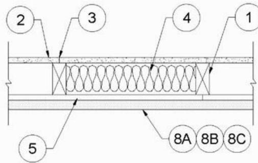
1. **Wood Studs** — Nom 2 by 4 in., spaced 16 in. OC in with two 2 by 4 top and one 2 by 4 bottom plates. As an option, nom 2 by 6 in., spaced 24 in. OC with two 2 by 6 top and one 2 by 6 bottom plates may be used in lieu of 2 by 4 studs and plates. Studs effectively fire stopped.
