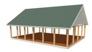
The default floor structure for a new room is a framed platform with wood flooring. This can be easily changed to a slab, or to no floor platform whatsoever.
