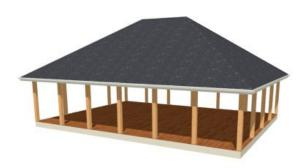
By default, the program will generate a roof plane over each exterior wall, producing a hip roof.
