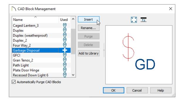
3. With the CAD block selected, click the **Insert** button, then click somewhere in the drawing area to place a copy of the selected CAD block.
