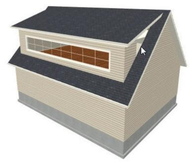
Notice there are small gaps in the dormer side walls. This gap is caused by the difference between the position of the knee walls, and the point at which the ceiling intersects the roof plane. This location is marked by the black dotted line in floor plan view.
