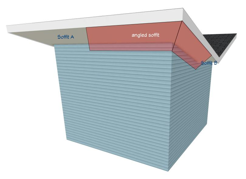
I can make the sloped soffit on soffit A with a polyline solid or molding polyline, but cannot do the same on soffit B because I can't get a PS to slope in two directions. I also tried a shadow board, but it has similar issues.
