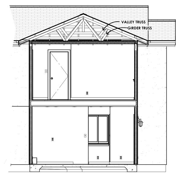
GRAPHICAL ROOF FRAMING REFERENCE NO SCALE
