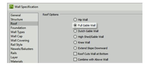
$\circ~$  On the Roof panel of the Wall~Specification dialog, select Full~Gable~Wall and
