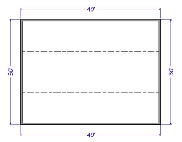
These are ceiling break lines, which represent the division between the flat, full height ceiling in the center of the room and the low, sloped ceilings on either side. The area with the flat, full height ceiling is loft area that will be accommodated by the open space at the center of your attic trusses.
