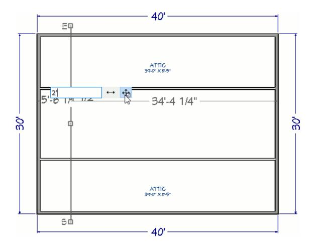
In this example, the truss is placed 24" from the outside of the wall's framing.
