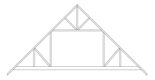
In order to create an attic truss, certain conditions must be met in the plan:
