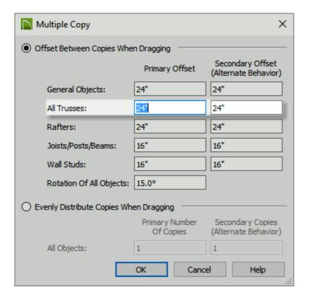
The **Primary Offset** is the interval at which trusses will be replicated when **Multiple Copy** is used. In this example, the default value of **24"** is used.
